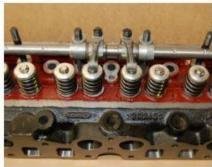
3.3 – Install rocker No.5, new spacer, and rocker No.4. There are no original washers used here. Then fit pedestal No.2.
