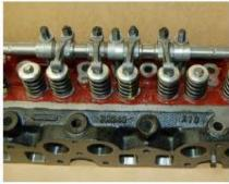
3.4 – Install rocker No.8, new spacer & rocker No.9. Again, there are no original washers used here. Then fit pedestal No.5.
